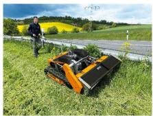
Image 1, Image 2: With the new flail mower AS 1000 Ovis RC, safe mowing is no problem even on extreme steep slopes up to over 50 degrees.
